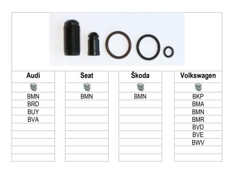
Always replace the adjusting screw as well when exchanging the ball pin. The Elring seal kit, injection nozzle 🥯 690.170 contains both components for this purpose. In addition to resulting in far greater wear, the use of an old and worn adjusting screw together with a new ball pin vastly increases the risk of ball pin fracture. Please avoid fitting an old adjusting screw in combination with a new ball pin.
